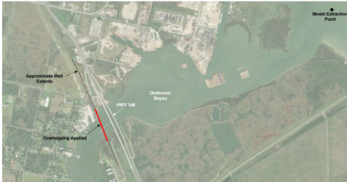
Figure 36. Model extraction point and representative wall length where overtopping was applied (red). Approximate wall extents also shown (black).
