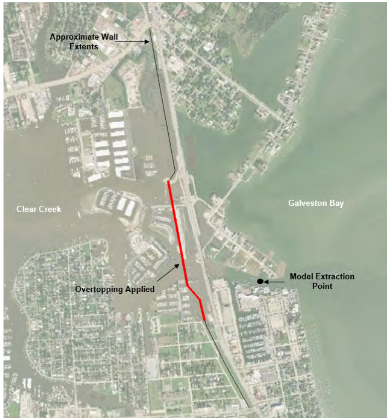
Figure 19. Model extraction point and representative wall length where overtopping was applied (red). Approximate wall extents also shown (black).
