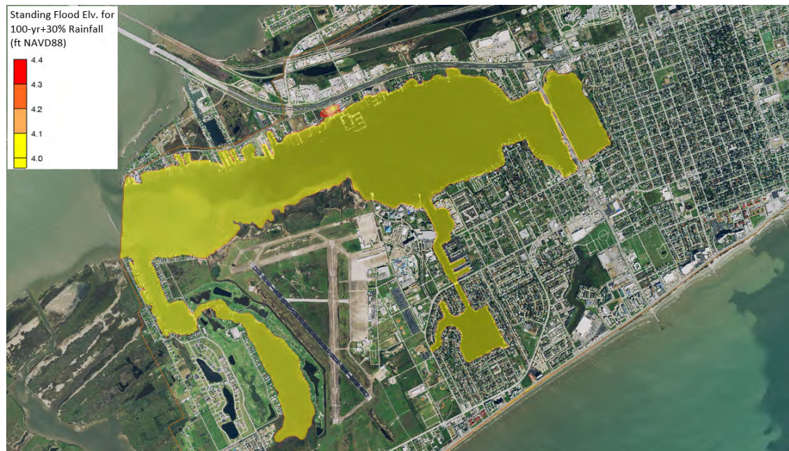
Figure 52. Standing flood coverage at elevation 4.4 ft NAVD88 from the 100-yr+30% rainfall with the 25-yr+30% facilities.
