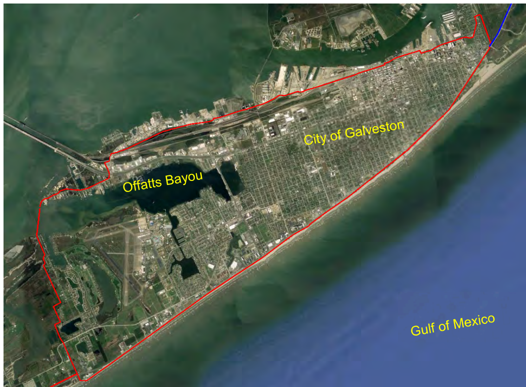
Figure 37. Figure of the proposed flood control alignment (red line) around Galveston as of November 2017.
