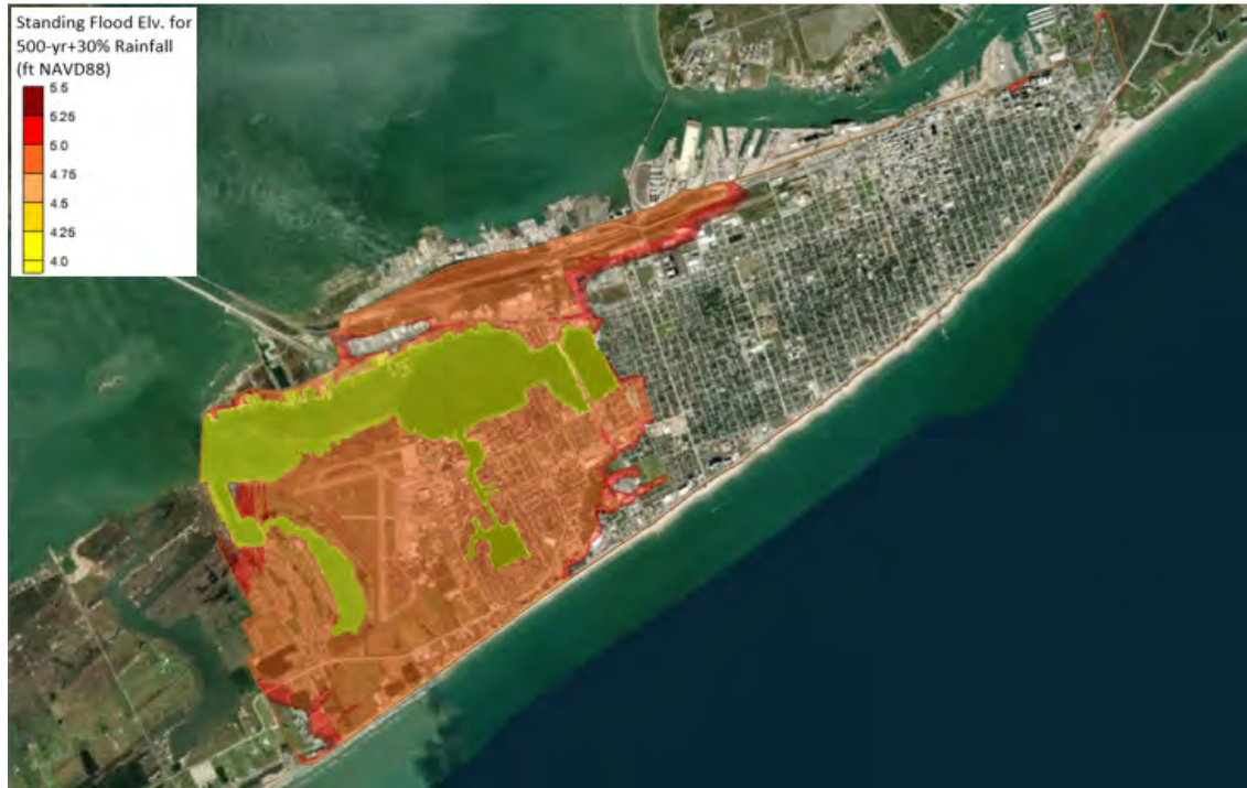
Figure 53. Standing flood coverage at elevation 5.5 ft NAVD88 from the 500-yr+30% rainfall with the 25-yr+30% facilities.
